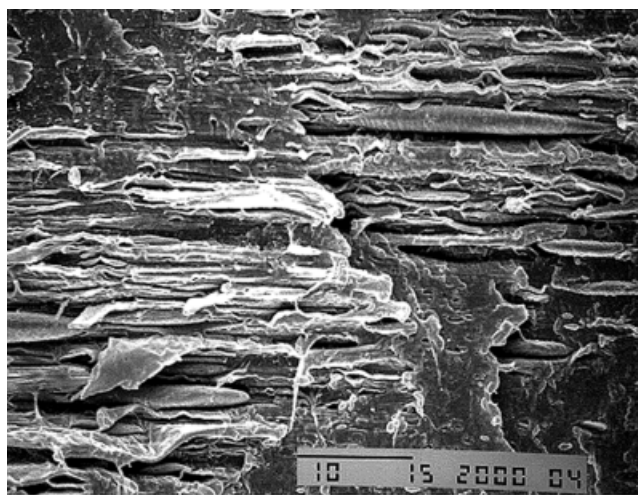
Figure 4 SEM micrograph of the surface of an oriented extruded film of a 75%/25%/4 pph R-PET/R-HDPE/EGMA blend. The draw ratio of the film was 3.5, and the surface was exposed by fracturing in LN 2 along the drawing direction.
